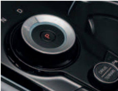
Quick-shifting electronic Shift By Wire (SBW) technology and standard Drive Mode Select (DMS) that adjusts transmission, throttle, and steering response.
