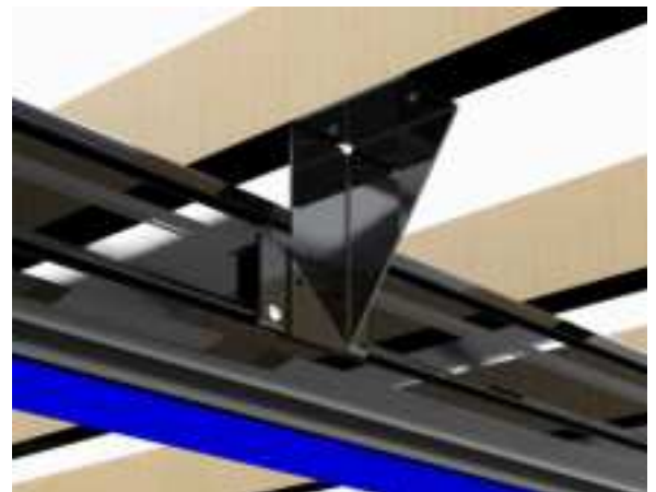
Figure 15: Cabaret case extrusion hanging off of ceiling mount
