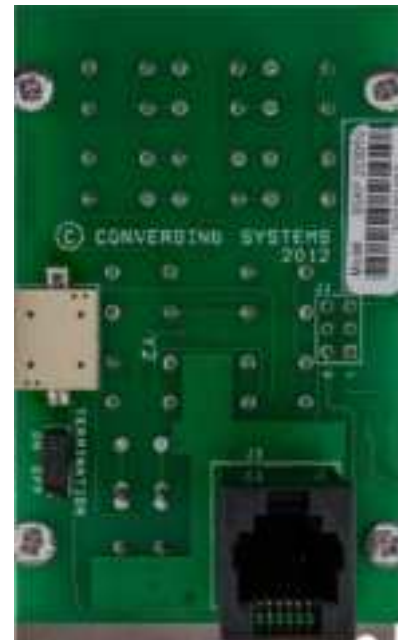
Figure 30: Rear of IR wall switch with RJ25 input
