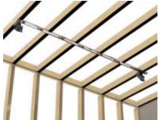
Figure 14. Ceiling brackets screwed onto ceiling joists
