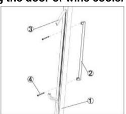
① Reveal two small holes on the door frame from inner side by pulling out a bit the door seal ② Aim the handle to the holes and insert the screws from inside ③ Screw them up with screw-driver ④ Put back door seal to cover the screws.
