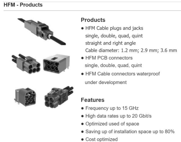
Figure 39: Description of the HFM Connector
