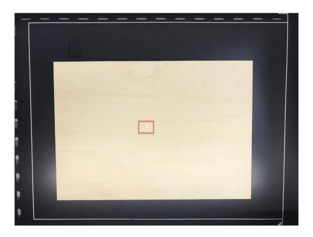
If the camera doesn't capture the material, you can open the lid and then close it to refresh the image, or click **Photograph** to refresh the image.
