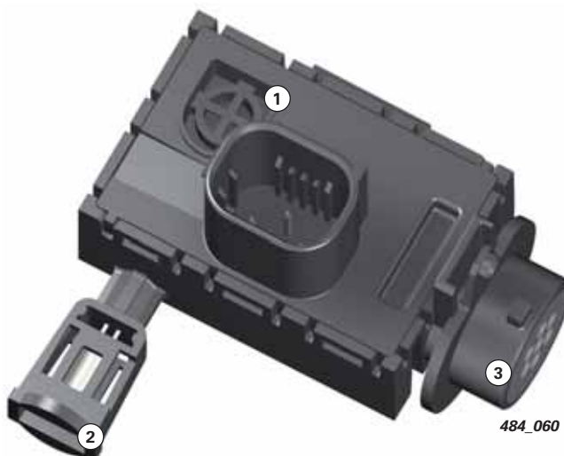
Humidity Sensor in Fresh Air Intake Duct G657 with Air Quality Sensor G238 in the four-zone climate control system
