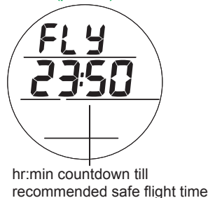
GAUGE STANDBY MODE (post dive)
