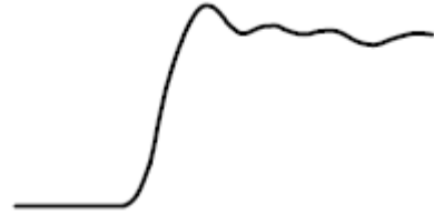
Long ground lead
