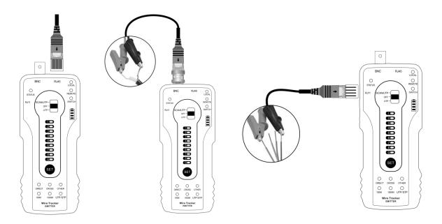
(1) Adjust the switch of emitter to the "Scan/UTP" mode, press "SET" key to switch to UTP/STP mode. The green light of the "UTP/STP" indicator means normal mode, while the red light is shielded mode. Turn on the wire receiver at the same time to trace the wire.
