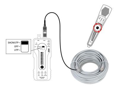
(2) Rotating the knob of receiver to adjust the sensitivity. When the cables are very close, can adjust to the small sensitivity to find the cable.
