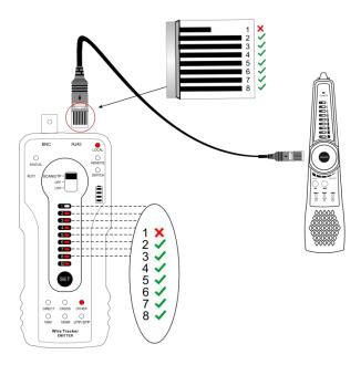
Under UTP mode, press "SET" key to switch to the "REMOTE" function
