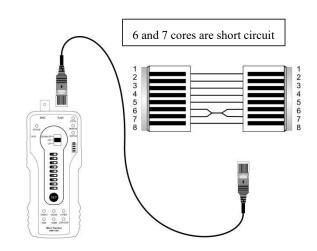
Emitter and Remote mode: The indicator lights of the short circuit pairs are flashing.
