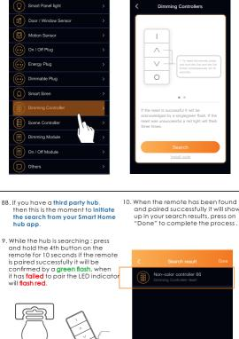
and hold the 4th button on the remote for 10 seconds if the remote is paired successfully it will be confirmed by a green flash, when it has falled to pair the LED indicator will flash red.
