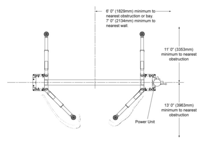
NOTE: Lift can be installed so power unit column can be located on either side. However, to save operation steps it is recommended that it is placed on passenger side of lift.
