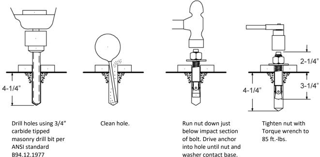
**STEP 10.** Using a level, check column for side-to-side plumb and front-to-back plumb. If needed, use horseshoe shims provided by placing shims underneath the base plate and around the anchor bolt. This will prevent bending the column bottom plates (Shim thickness should not exceed 1/2"). Tighten 3/4" anchor bolts to **85 ft-lbs.** of torque.
