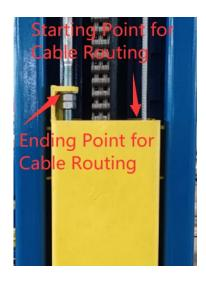
For cable routing start at the rear right, passed around the down pulley (rear to front). Then travels back up and across to the opposite column.
