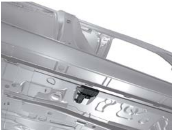
Front Passenger Access/Start Antenna R135. On body under 'B' pillar area.
