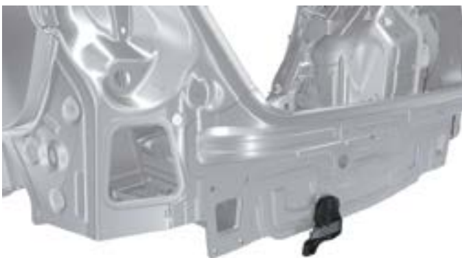
Access/Start System Antenna in Rear Bumper R136.
