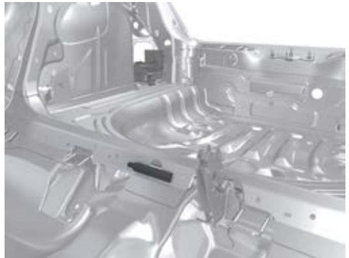
Access/Start Antenna in Luggage Compartment R137. Located under seat.
