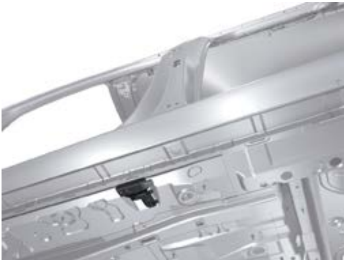
Driver Access/Start System Antenna R134. On body under 'B' pillar area.
