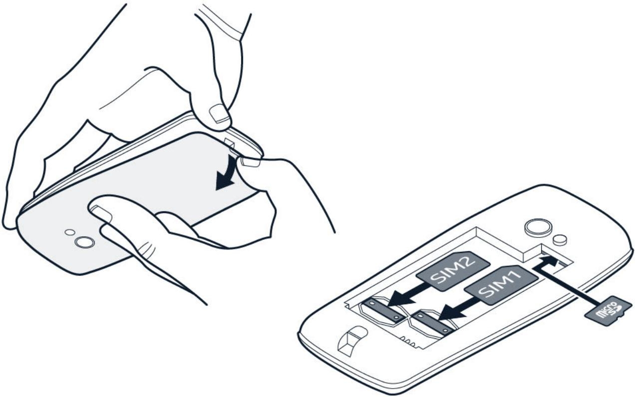
1. Put your fingernail in the small slot at the bottom of the phone, lift and remove the cover.
