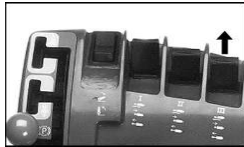
Figure 20: SCV III Pushed Forward
