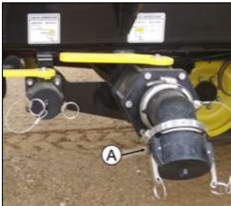
A. Main Tank Fill Line
