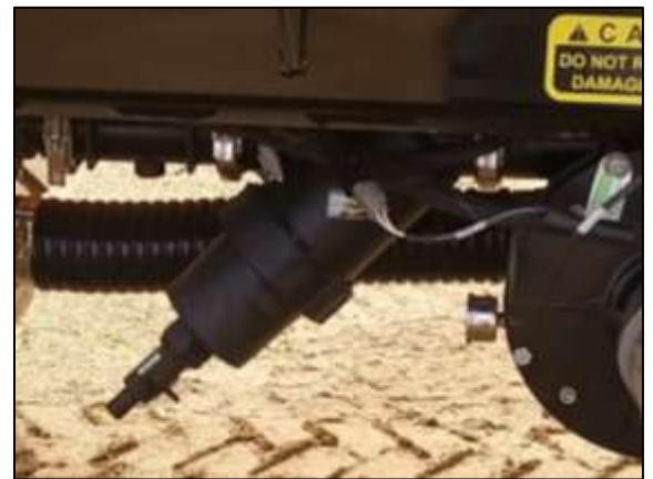
Figure 25: Pump line feed filter/strainer
