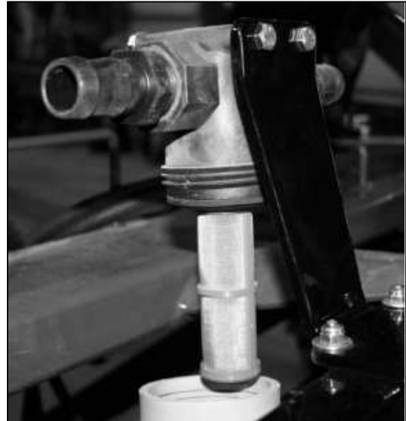
Figure 24: Typical boom line filter/strainer
