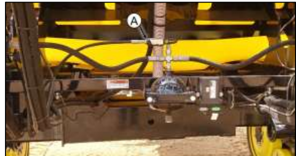
Figure 12: Boom lift shutoff valve above accumulator
