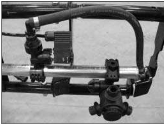
Figure 3: Electric shutoff fence row nozzle
