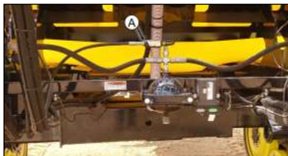
Figure 12: Boom lift shutoff valve above accumulator
