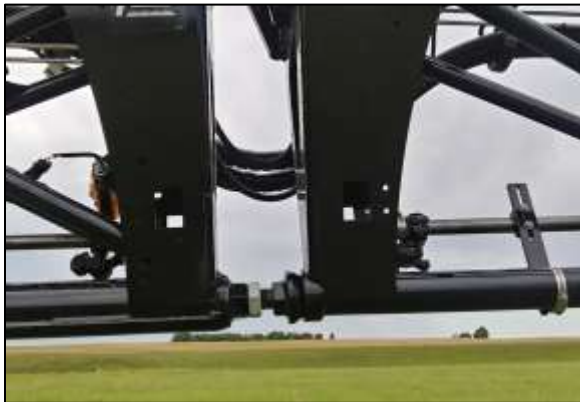
Figure 26: Inner boom adjustment bolt
