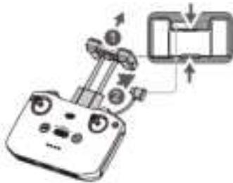
3. Place the mobile device onto the mobile device holder, and plug the RC cable into the mobile device.
