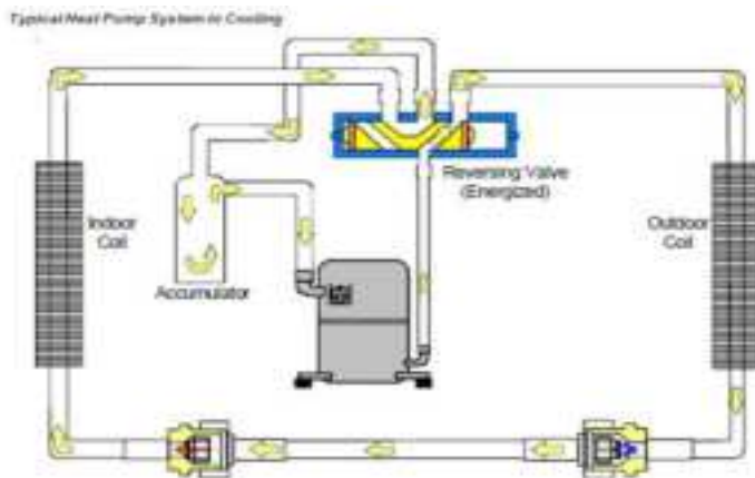
FIGURE 8: HEAT PUMP COOLING SCHEMATIC
