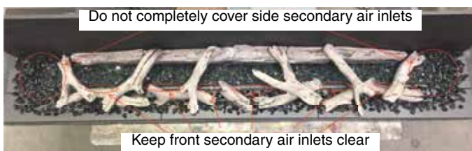
Correct Black Coal placement - Driftwood logs shown
