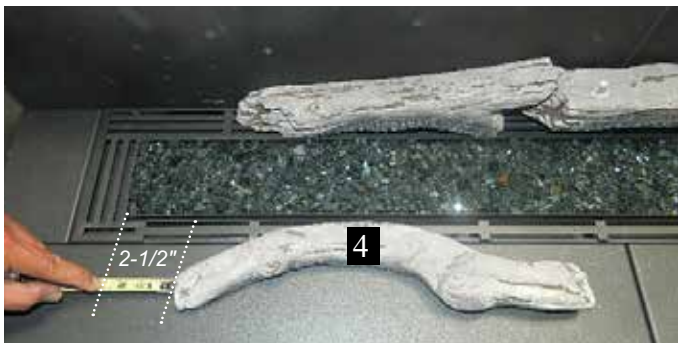
Log 4 to edge of burner
