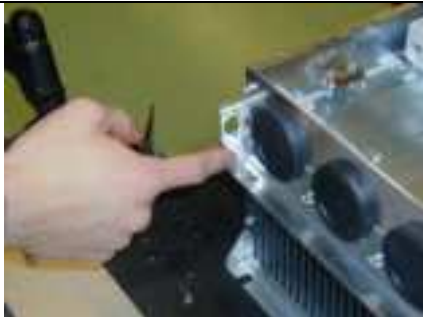
10. Smoothen all sealed seams with your finger. Tip your finger in soap water before smoothing the seams.
