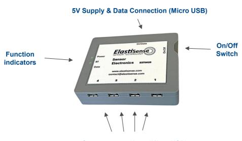
Sensor connections (Micro USB)
