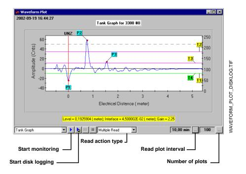
The **Read Plot Interval** entry field specifies the time interval between plots that are saved to disk. For example, type 10 if you want the waveform plot to be updated every ten minutes.
