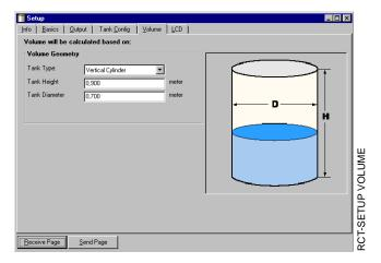
You can choose one of the standard tank shapes or the strapping option. Choose None if volume calculation is not used at all.
