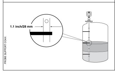
Coaxial probe fixed to the tank wall.
