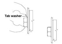
4. Secure the bolt by folding the tab washer.
