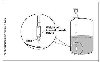
Flexible Twin/Single Lead probe with weight and ring.
