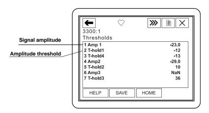
2. Open the desired amplitude threshold for editing.
