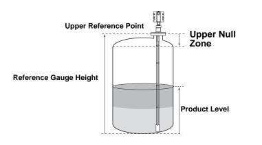
Figure 6-9. Identifying the Upper Null Zone in the RCT Waveform Plot
