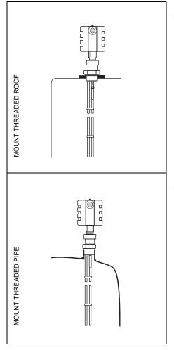
Mounting on tank roof.
