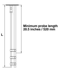
2. Update the transmitter configuration to the new probe length, see "Probe Length" on page 4-9.
