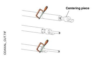
To cut a coaxial probe do the following:
