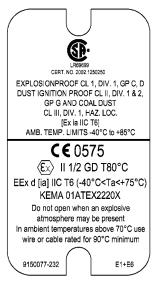
Figure B-7. Approval Label CSA Explosion-Proof and FM Explosion-Proof.
