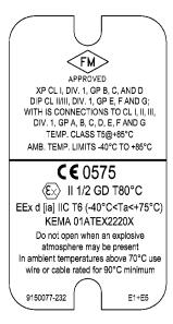
Figure B-9. Approval Label ATEX Intrinsic Safety and CSA Intrinsic Safety.
