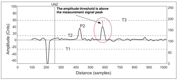
Figure 6-4 illustrates a situation where amplitude threshold T3 is too high. The signal amplitude peak at the interface between the upper and lower products is not detected in this case. By adjusting amplitude threshold T3, the peak at the interface between the upper and lower products is detected as illustrated in Figure 6-5:
