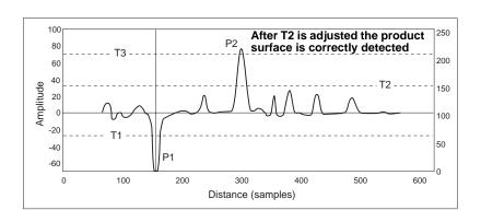
To adjust the amplitude thresholds select HART command [1, 4, 5, 3] or
