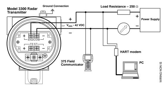
For HART communication a minimum load resistance of 250 Ohm within the loop is required. For maximum load resistance see Figure 3-12 (Explosion/Flame Proof) and Figure 3-13 (Non-hazardous installations).
