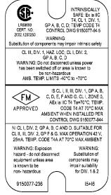
Figure B-11. Approval Label ATEX Intrinsic Safety and FM Intrinsic Safety.
