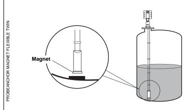
**Flexible Twin/Single Lead** probe with weight and magnet.
