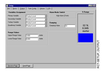
Typically, the **Primary Variable** (PV) is configured to be Product Level, Interface Level or Volume.
