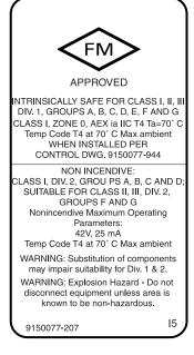
For connection in ambients above 70 °C, use wiring rated for 90 °C
