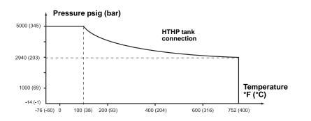
Figure A-3. Process temperature and pressure diagram for HP tank connection.
