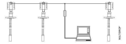
The poll address can be changed by using a 375 Field Communicator or by using the Rosemount Configuration Tools software.
