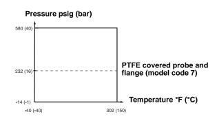
Figure A-2. Process temperature and pressure diagram for HTHP tank connection.
