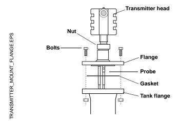
Figure 3-10. Tank connection with loose flange ("plate design").
