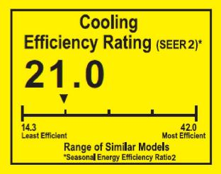
This system's efficiency ratings depend on the coil your contractor installs with this unit. The heating efficiency rating varies slightly in different geographic regions. Ask your contractor for details.
