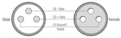
Resistance 120 ohm // ¼ w between pin 2 (DMX-) and pin 3 (DMX+) oft he last fixture.
