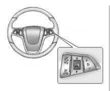
(Mute/End Call): Press to decline an incoming call, or to end a current call. Press to silence the vehicle speakers while using the infotainment system. Press again to turn the sound on. Press to cancel voice recognition.
