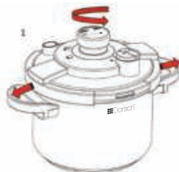
1. Press down the knob lightly and turn the knob towards the unlocking symbol
