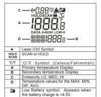
Figure 3. Thermometer Display
