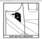
The Dust Bin Full indicator will illuminate when the dust bin is full of debris and needs to be emplied. To reset the indicator, remove the dust bin and empty it.
