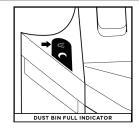
The Dust Bin Full indicator will illuminate when the dust bin is full of debris and needs to be emptied. To reset the indicator, remove the dust bin and empty it.
