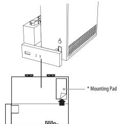
\* Peel off the film that is on top of the mounting pad that will help to secure the Side Dock Charging Station to the Xbox Series S. 3 Carefully place the Xbox Series S console on it's side. Slide the locking switch on the Side Dock Charging Station to fasten it to the bottom of the console.
