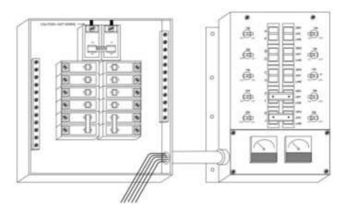
6. Trim the supplied conduit to the desired length and slide over the VEVOR transfer switch wires. Attach to the fitting on the VEVOR transfer switch.
