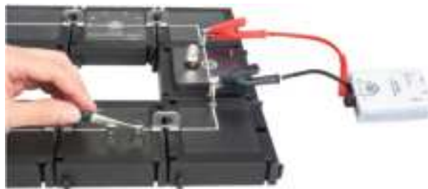
Figure 1: The Wireless Voltage Sensor connected in parallel to a circuit.
