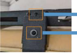
bolt first, and then tighten the lower bolt.
