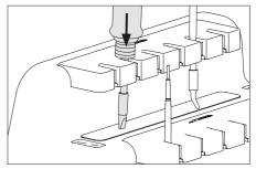
To insert the cartridges, place the handle on top of the new cartridge and press the handle down slightly.
