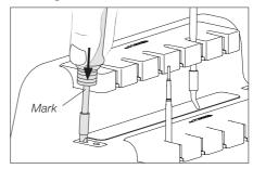
Use the hole that best fits to the cartrige tip dimension and push the handel down as far as the mark on the cartridge\*.
