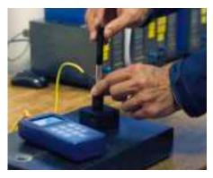
Push down the sleeve to 'load' the probe and prepare for testing.
