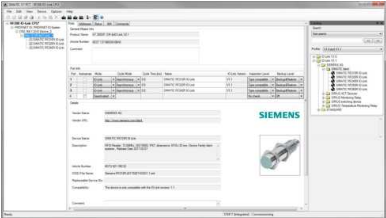
Figure 5-3 Creating IO-Link master ports
