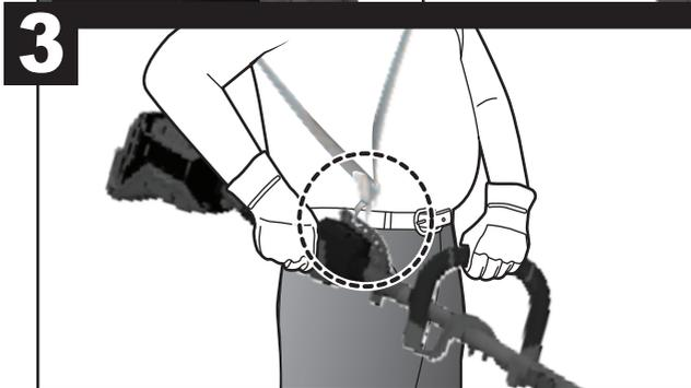
**NOTE:** Adjust the harness so that the height of the product is level with the hips.
