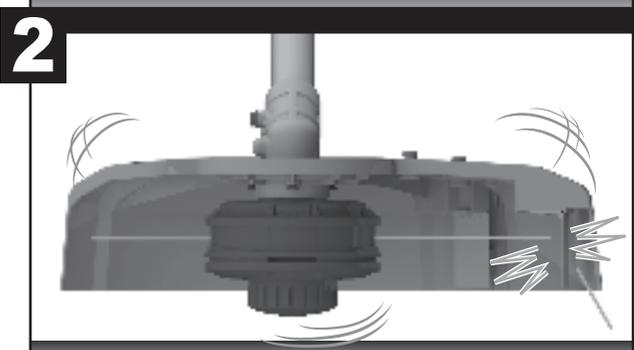
**NOTE:** The cut-off blade automatically trims the newly extended line to the correct length for safe and optimum performance.
