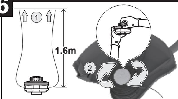
**NOTE:** When using the 2.4 mm line, the total line length should be 3.3 mm or 1.6 m visible line on each side.
