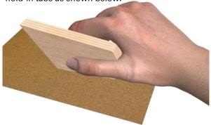
**4.** Round all the edges of each fin, except the root edges. Leave them flat. Repeat for all six fins. The root edges will be glued to the body tube.
