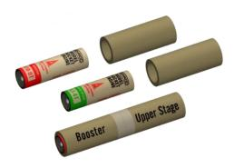
■ **25.** Insert the "booster" end of the engine assembly into the top of the booster section. Then insert the "upper stage" engine into the bottom of the sustainer section. Apply a few sheets of recovery wadding in the top of the main body tube. Fold the streamer and pack it and the shock cord on top of the recovery wadding. Slide the nose cone into place, making sure it does not pinch the shock cord or streamer.
