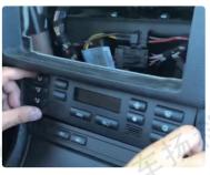
2 Connect the new radio wires to the original car wiring, gently lift the air vent, and insert the new radio frame into the corresponding position.
