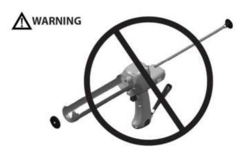
Never remove the push rod off the tool in any case, otherwise it will cause failure of spheres locating which makes the gun fail to work.
