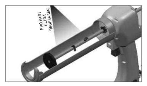
In case of residual material left on the push rod, please clean it up thoroughly before pulling the rod to the backward position. The purpose is to prevent the material from entering the inner mechanism and keeping the tool in good condition.
