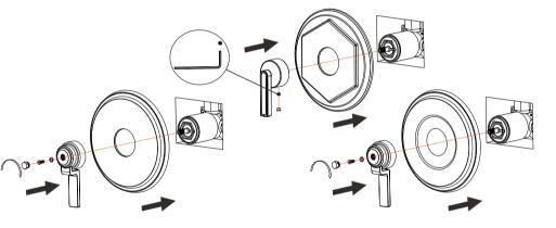
6.Aftet installing the plate, install the handle.
