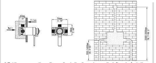
1.Cut the groove on the wall according to the dimensions on the left, and refer to the dimensions on the right.
