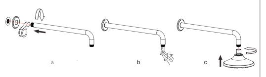
7.Installation of shower arms(a), flushing of pipes(b), installation of overhead spray(c).
