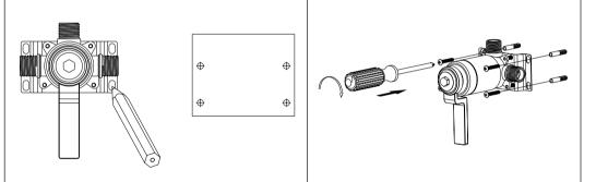
2.Mark the position with a marker and punch the holes.
