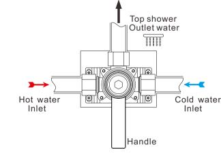
4. Connect the water pipe(pay attention to the direction of hot and cold water)
