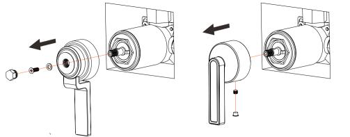
5. Remove the handle before installing
