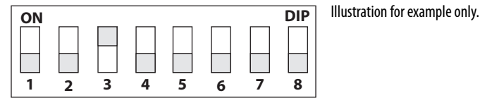
Figure 57 - Drive Size DIP Switch S15 Example
