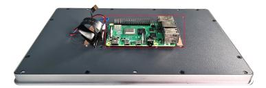
5. Pass the FPC cable through the reserved hole on the ED-Pi4PCOOLER.
