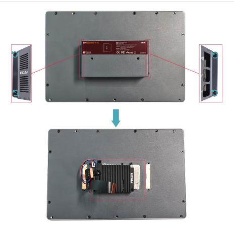
3. Use a screwdriver to loosen 3 M2.5 screws on ED-Pi4PCOOLER counterclockwise, and remove the cooler.
