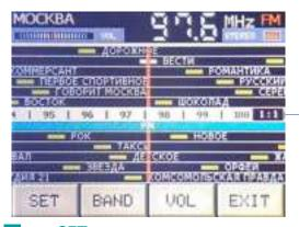
The SET button is used to calling additional buttons.
