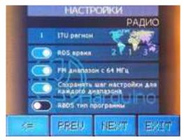
The <= button is used to calling additional buttons.
