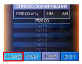
The CHANGE button is used to calling additional buttons.
