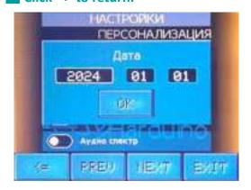
To enter setup mode, press the SETUP button on the main screen. Settings are divided into pages. Switching pages is done by rotating the encoder or using the PREV and NEXT buttons. Click WIFI for connection settings (page 15). Press RESET to load default settings. To save settings, press SAVE or EXIT and confirm saving.
