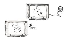
When moving the television to a warm location from a cold location, allow some time for any dew or condensation inside the television to evaporate fully before you turn the unit on.
