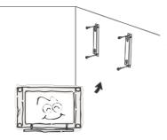
To prevent injury, the television must be securely attached to the floor/wall in accordance to the supplied installation instructions.
