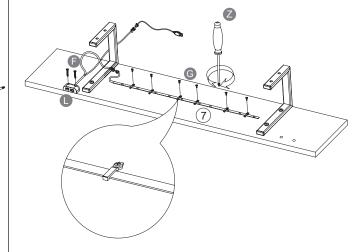
Please attach the  $\bigcirc$  cable clips according to the arrows. Tighten the  $\bigcirc$  LED light and  $\bigcirc$  USB Cable and fasten the cable clips.
