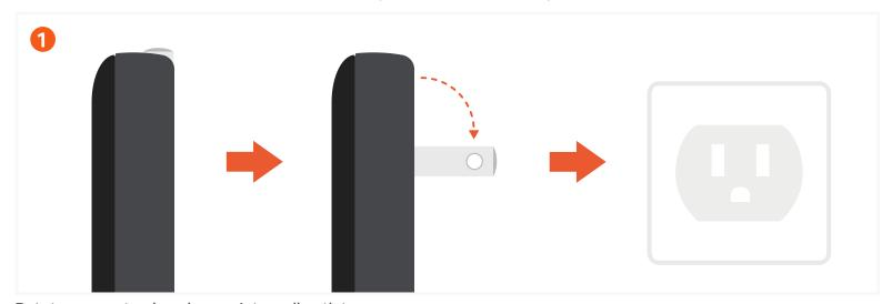
Rotate prongs to plug charger into wall outlet.
