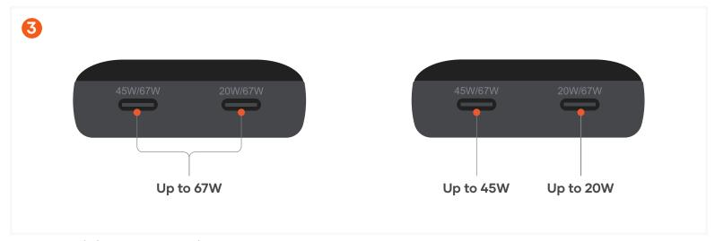
Connect and charge up to two devices at a time:
