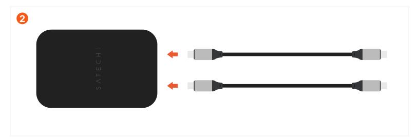
Insert a USB-C cable into charger's USB-C port (cables sold separately).
