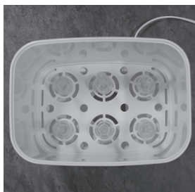
FIGURE D. Placement of wide-neck reservoir tubes
