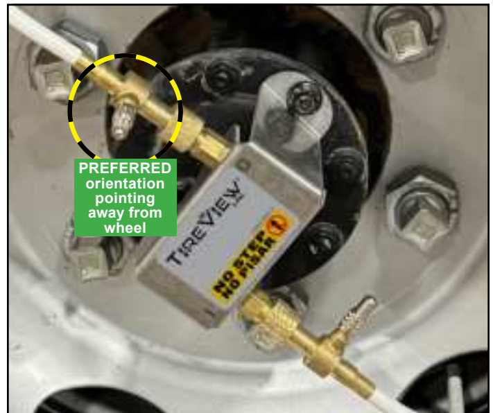
Figure 10: Correct orientation of check ports.
