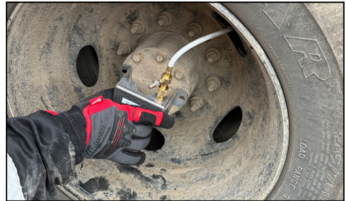
Figure 6: Determine bracket mount location.
