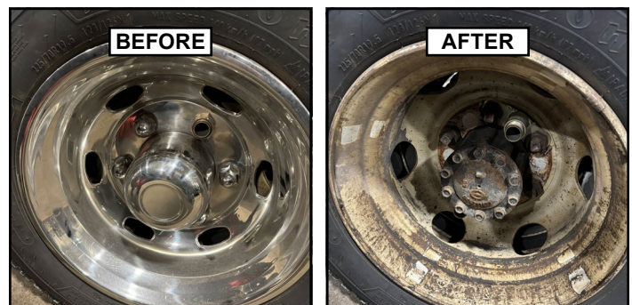
Figure 8: Cosmetic wheel coverings must be removed.
