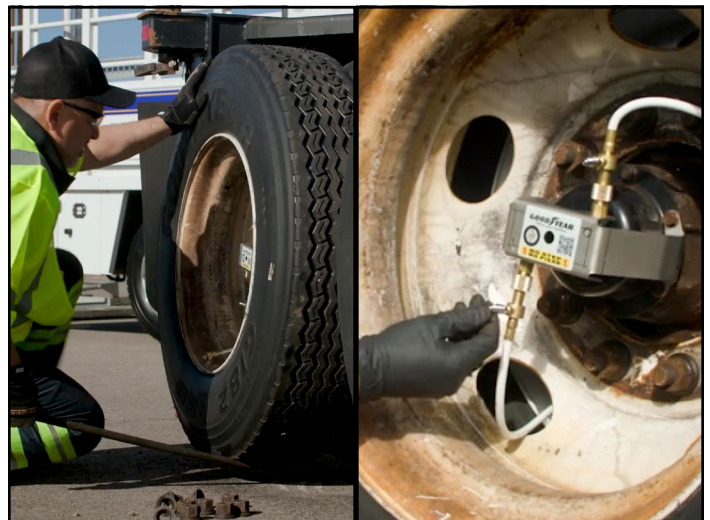
Figure 17: Reinstall over hub & bracket and reinstall hoses.
