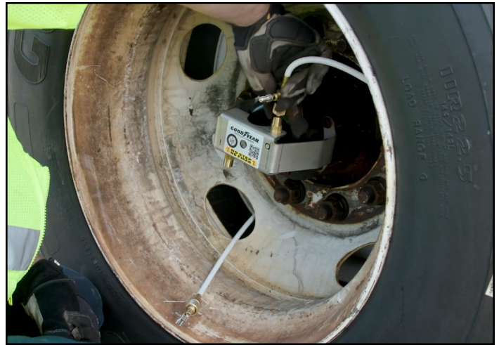
Figure 14: Remove hose(s) from bracket.
