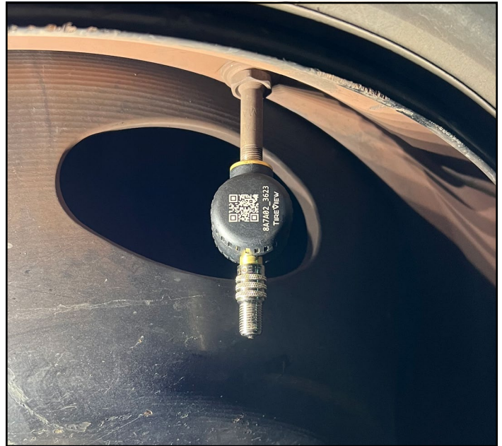
Figure 13: Front steer flow-thru sensor installed.
