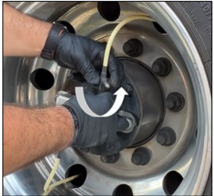
Figure 9: Hand-tighten knurled hose fittings.
